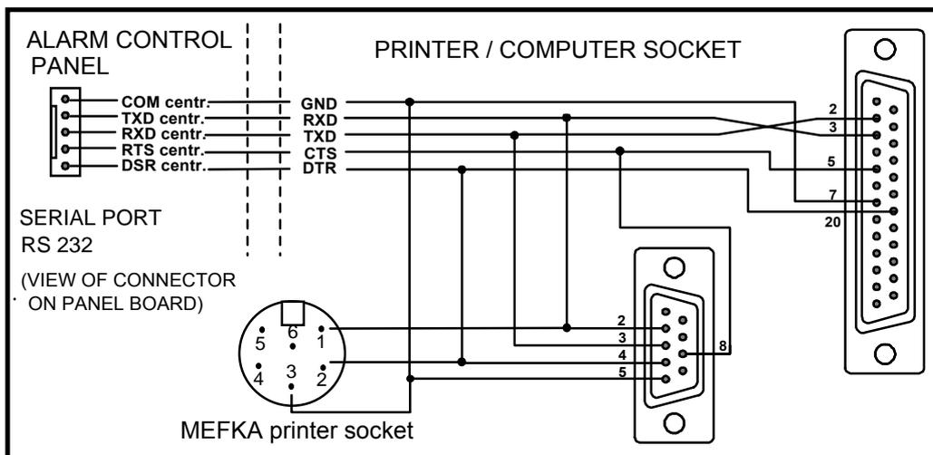
*Fig. 11 - Connection of printer or computer to panel RS-232 port.*
