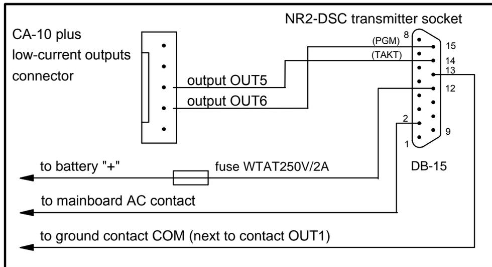
Figure 9 - Connection of NR2-DSC controlled transmitter, made by NOKTON s.c.
