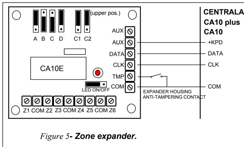
The jumpers A, B, C, D are used for setting the expander address – the upper position corresponds to a jumper set in the keypad. The jumpers C1 & C2 should be set as required by the number of keypads connected to the panel. The expander jumpers must be set in either upper or lower position - they must not be permanently removed.
