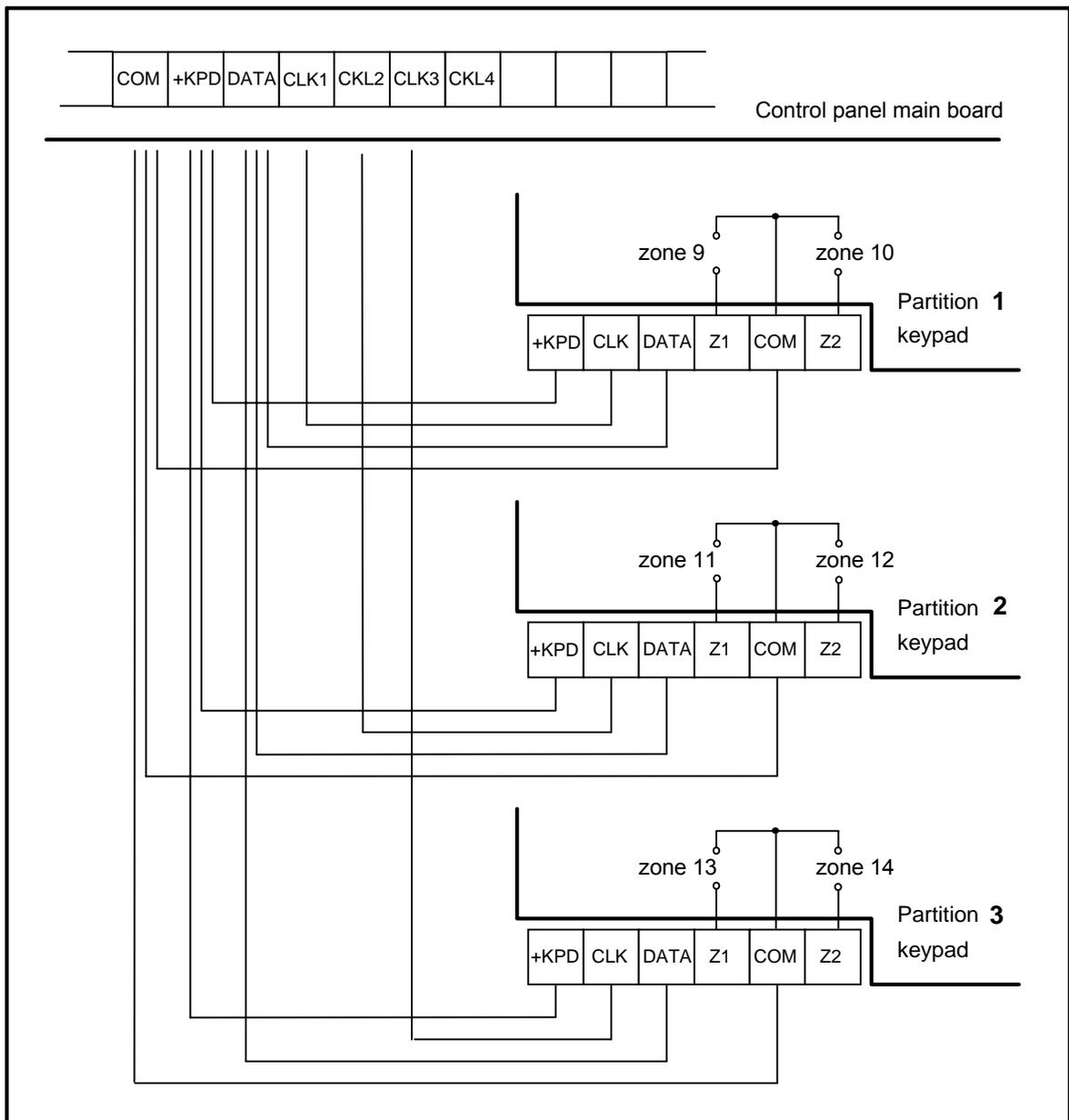
Figure 4 - Connection of three keypads to the control panel.
