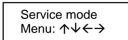
Pressing any arrow key will display the service mode **hierarchical menu**, which facilitates access to the service functions. The menu is built so as to group the particular panel service functions by subjects.
