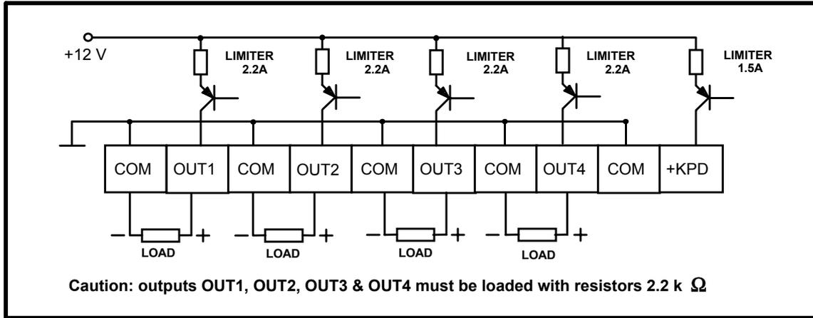
Figure 7 - Diagram of high-current outputs.
