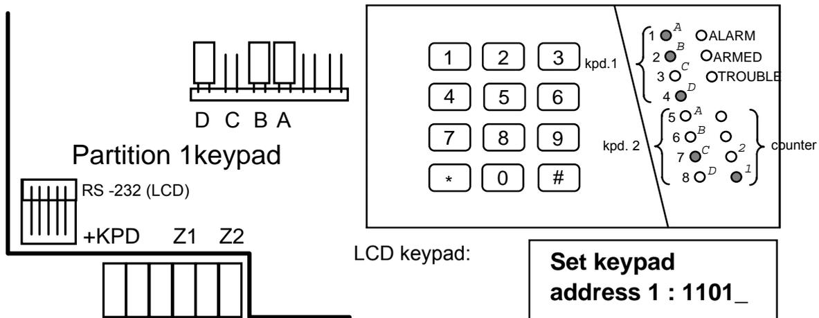
Fig. 14 - Jumper setting and corresponding LEDs during programming.
