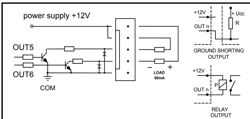
Figure 8 - Diagram of OUT5, OUT6 low-current outputs and load connection.
