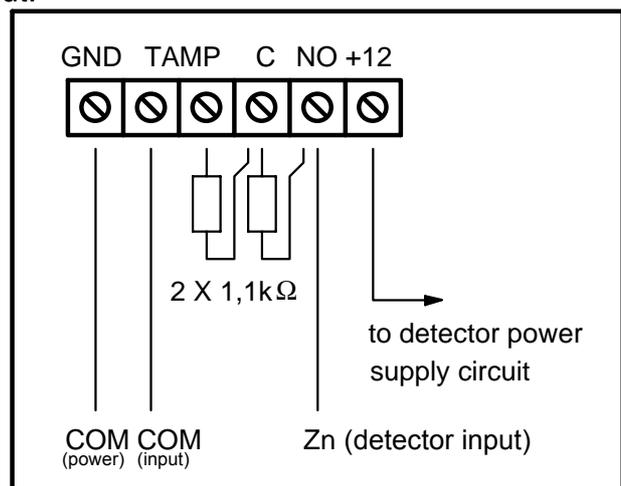
Figure 6 - Connection of 2EOL detector.
