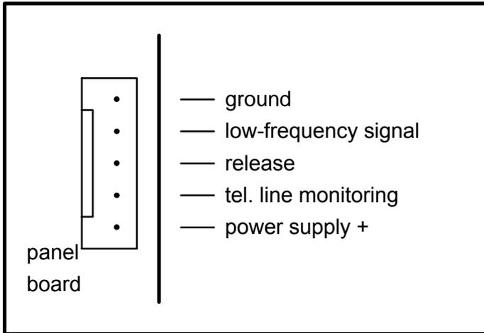
The CA-6 plus panel interfaces with the SM-2 synthesizer. The synthesizer socket (designated as: SM-2 VOICE SYNTHESIZER) is situated on the right-hand side of the printed board, between the telephone line connector and the socket of OUT5, OUT6 outputs. The SM-2 synthesizer should be directly plugged into this connector. It is fitted with minijacks for playback of the message and "monitoring" of the telephone line.
