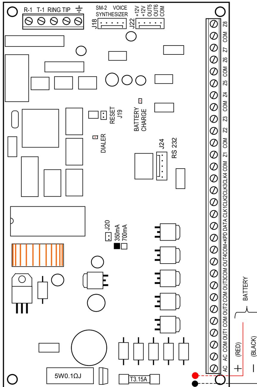
Figure 1 - Diagrammatic view of control panel main board, version CA10PV4.3.
