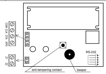
Figure 2. Schematic view of the keypad board including designations of wire terminals (version LCD-S V1.6).
