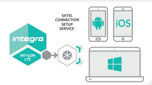
Communication with the control panel via the **INT-GSM LTE** module can take place through the SATEL connection setup service. This makes it possible to remotely:
