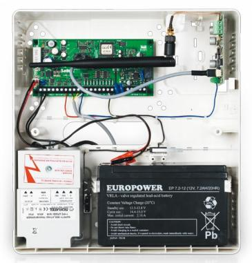
an example hardware configuration in the **OPU-4** housing
