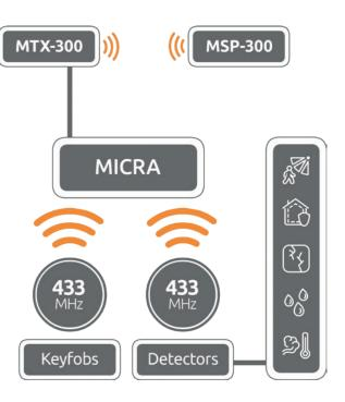
The MTX-300 can also be connected to the MICRA module to extend its functionality by adding capability to control the MSP-300 wireless sirens. Wired inputs of the module can be used to receive signals from an increased number of detectors. As a result, the MTX-300 makes it possible to use up to 12 wireless detectors in the system or expand it by adding extra keyfobs.
