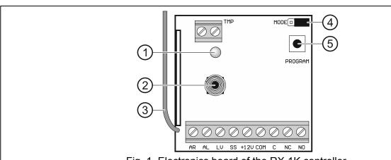
Fig. 1. Electronics board of the RX-1K controller.
