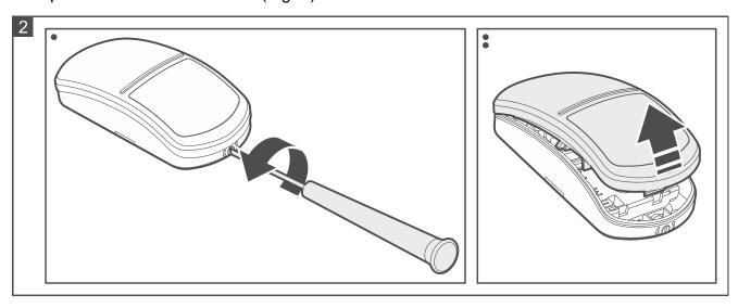
2. Press the catches and move the electronics module down, then remove it from the enclosure base (Fig. 3).
