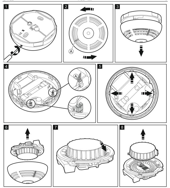
15. Press and hold down the test / reset button (designated with the letter A in Figure 2). Alarm should be triggered after a few seconds.
