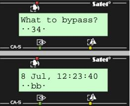
[#] -accepting the entered data - four short beeps and a long one signal end of the function.
