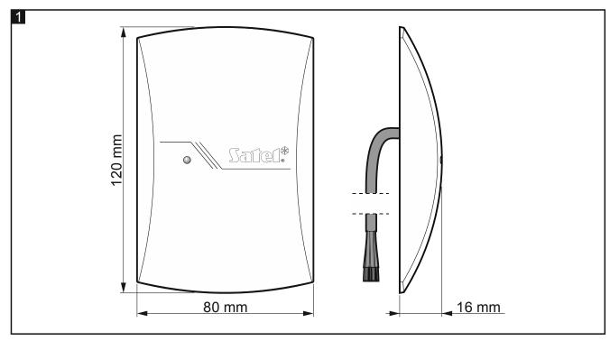
The electronic circuit is potted in epoxy resin for protection against moisture and dust. The multi-conductor cable is led-out of the reader enclosure.
