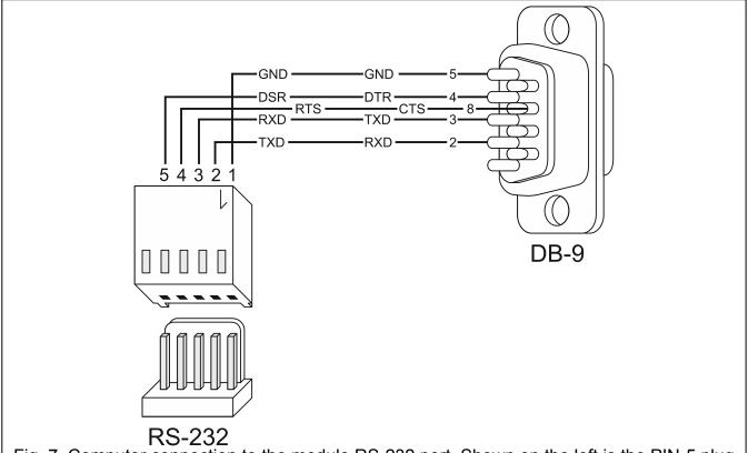
Fig. 7. Computer connection to the module RS-232 port. Shown on the left is the PIN-5 plug to be connected into the module connector. Shown on the right is DB-9 female plug (solder side view). A ready cable is offered in the DB9F/RJ-KPL set.
