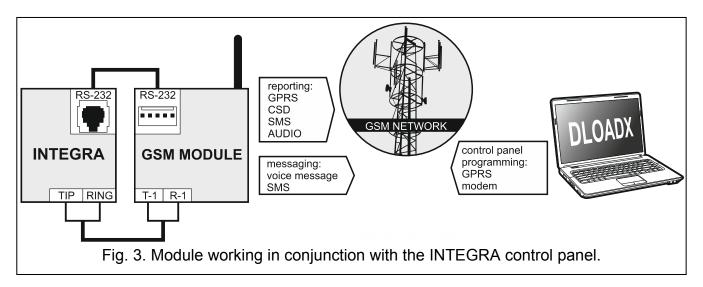
When connected to the INTEGRA control panel, the module offers the following benefits:
