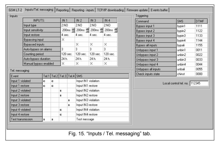
**Auto-bypass on alarms [49]** ... **[52]** – the number of input violations after which it will be automatically bypassed, after the module registers the end of last violation. Values from 0 to 15 can be programmed. Value 0 means no bypass.
