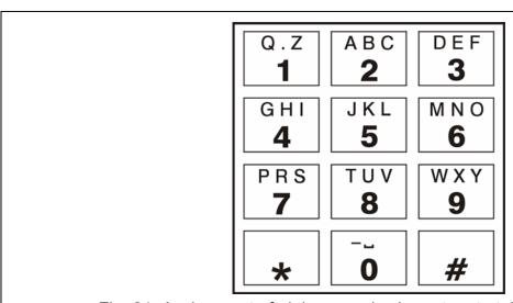
Fig. 21. Assignment of alphanumeric characters to telephone keypad.
