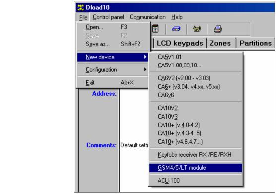
Fig. 8. Selecting the GSM module after starting the DLOAD10 program.
