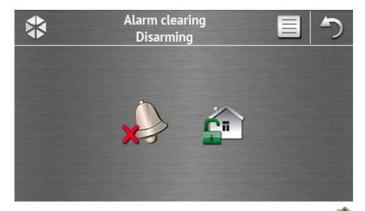
The "Alarm clearing / Disarming" screen will be displayed after you tap the icon on the main screen, when there is an alarm (alarm memory) and at least one partition is armed.
