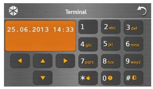
The terminal enables the alarm system to be operated and programmed in the same way as from the LCD keypad with text menu. The method of using such a keypad is described in the control panel programming / user manuals (electronic versions of the manuals are available on the www.satel.eu website).
