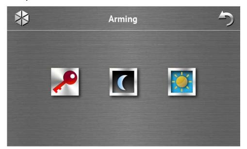
This screen is displayed when you can arm one partition only (also when the quick arming is allowed by the installer in one partition only).
