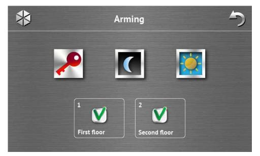
This screen is displayed when you can arm both partitions. The partitions are presented by means of appropriately described fields. By default, the  $\bigvee$  icon is displayed in both fields, which means that the partition is to be armed. Tap on the field, if the partition is not to be armed (the  $\bigcirc$  icon will be displayed). Having defined where the system is to be armed, tap one of the icons to arm the system.
