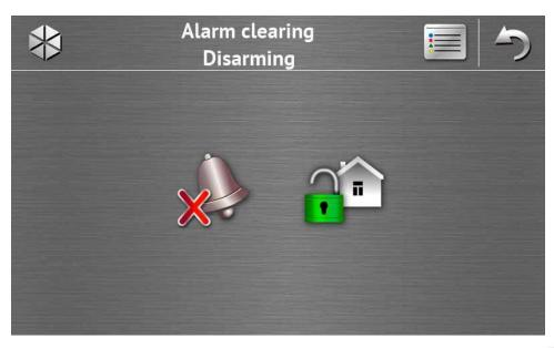
The "Alarm clearing / Disarming" screen will be displayed after you tap the **main** icon on the main screen, when there is an alarm (alarm memory) and at least one partition is armed.
