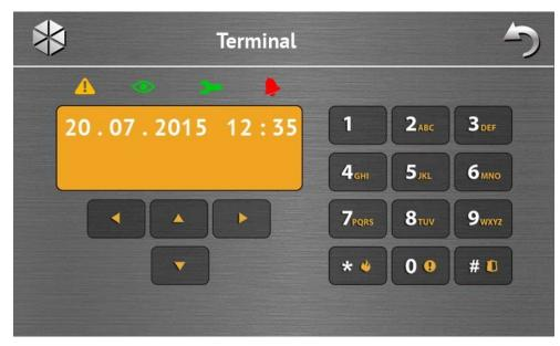
The terminal enables the alarm system to be operated and programmed in the same way as from the LCD keypad with text menu. The method of using such a keypad is described in the control panel programming / user manuals (electronic versions of the manuals are available on the www.satel.eu website).
