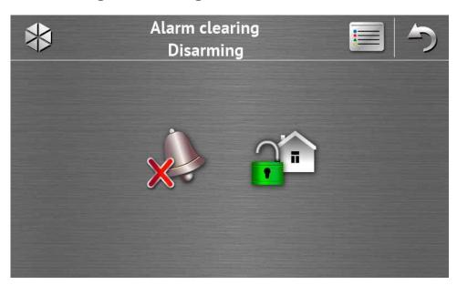
The "Alarm clearing / Disarming" screen will be displayed after you tap the icon on the main screen, when there is an alarm (alarm memory) and at least one partition is armed.
