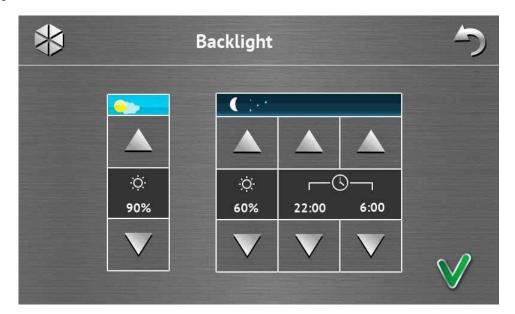
Intensity of the screen backlight can be controlled within the 10-100% range. In the night hours, which can be specified, the backlight intensity can be different.
