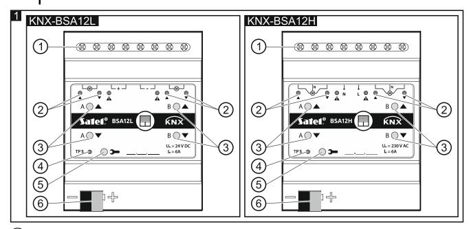
1 connecting terminals for blind/shutter motors and power supply.
