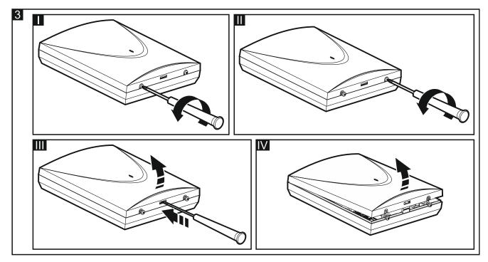
1. Loosen the cover locking screws and remove the enclosure cover (Fig. 3).
