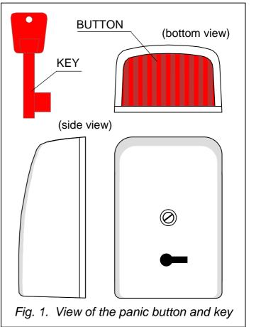
inside the casing until it is released with the key. Where a few buttons are connected to one zone of the alarm control panel, this function makes it possible to identify the button which triggered the alarm.
