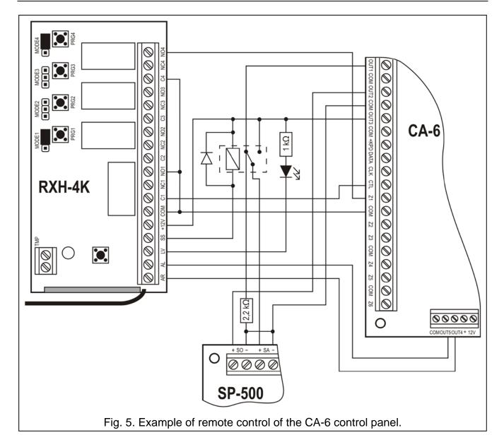
The SS output controls the relay, which supplies +12 V voltage to the +SA siren input and, consequently, generates a sound signal. The OUT1 control panel output remains connected via the 2.2 k $\Omega$  resistor to the common ground in the siren, thus ensuring presence of the load on the OUT1 output, as well as cabling control when armed/disarmed states are being signaled. The resistor should be installed inside the siren housing.
