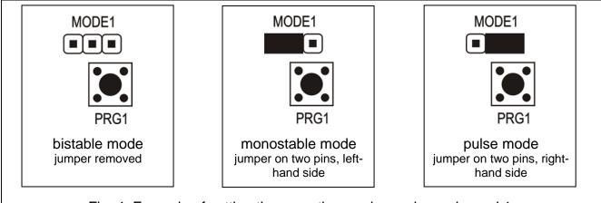
Fig. 4. Example of setting the operating mode on pins – channel 1.
