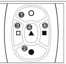
Fig. 5. MPT-300 (black enclosure) / MPT-350 (light gray enclosure) keyfob [433 MHz keyfob]. A – numeration of keyfob buttons (button 5 – pressing buttons 1 and 2 simultaneously).
