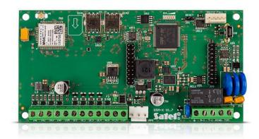
GSM-X offers sending notifications to 8 telephone numbers in several ways: by using voice, SMS or PUSH messages, or via the CLIP service.
