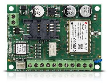
The module is provided with 5 programmable inputs, either digital (NO, NC) or analog. When configured as analog ones, the inputs can be used in automation systems, or for monitoring of a wide range of external devices, such as analog sensors of temperature, pressure and humidity.
